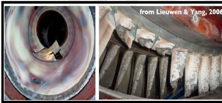
Figure 1: Damages on Combustor Liner and Turbine Blades by combustion Instabilities. Liewen and Yang (2006)
